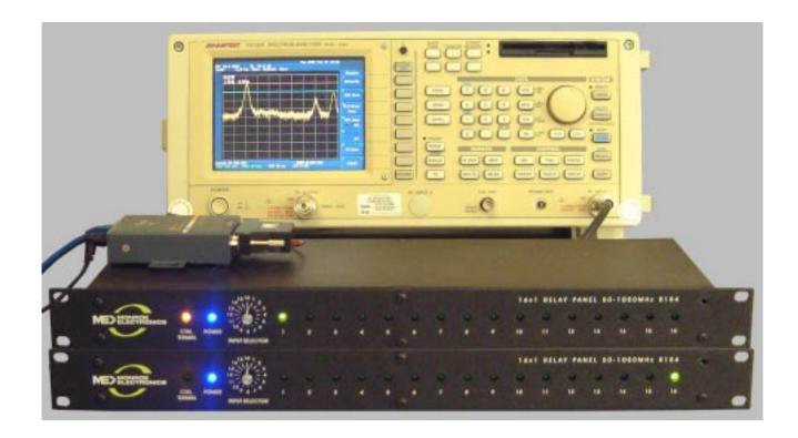
This is a picture of two units configured as a matrix connected to a spectrum analyzer.
