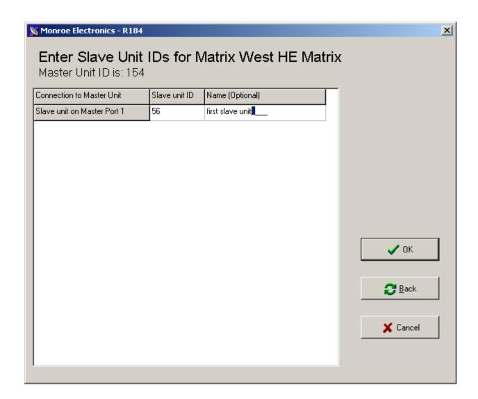
• Enter the Slave Unit id number, and enter a reference name for it. Once this is done, select OK, then click on Yes on the following screen to configure the matrix. This example shows the setting of a Matrix with one slave unit.
