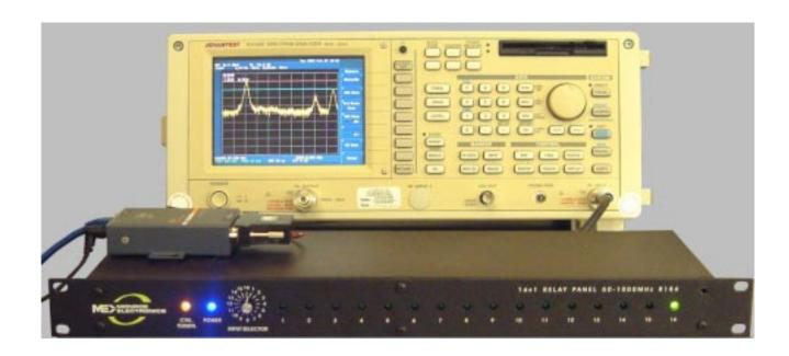
This is a picture of a single unit connected to a spectrum analyzer. Note that the orange LED indicates that the termination is set, since it is at the end of the RS485 connection. And that input 16 is being sent to the spectrum analyzer.
