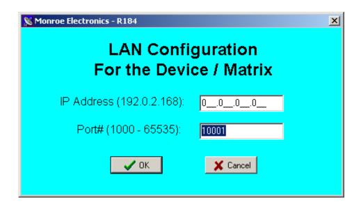
This screen permits input of the IP Address for the Ethernet adaptor being used, and the Port number it communicates through. These are noted on the R184/98 LAN to RS485 adaptor, and configured for your system by your IT personnel to allow the proper operation. The example below is set up for a system at Monroe Electronics.
